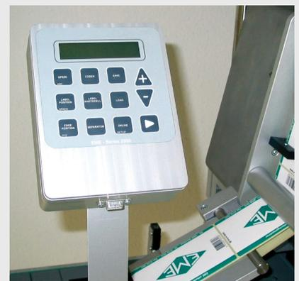
Separate key pad for operating the dispenser on distance. It can be mounted in any position within a distance of up to 5 meters from the dispenser.
